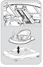
2 To adjust the height to the upper position, pull the upper tray to the height you require. To adjust the height to the lower position, turn the adjustment buttor 90 degrees and press the button upward to release the lock, then press the tray to the required position. Warning: Please make sure the
